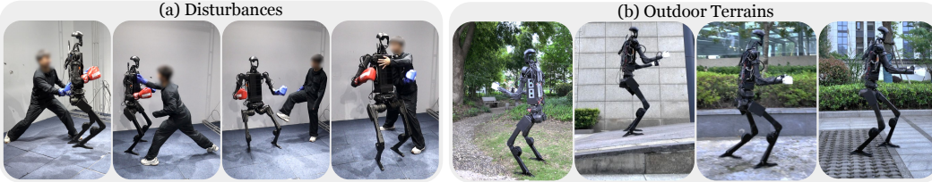
Figure 5: OmniH2O shows superior robustness against human strikes and different outdoor terrains.
